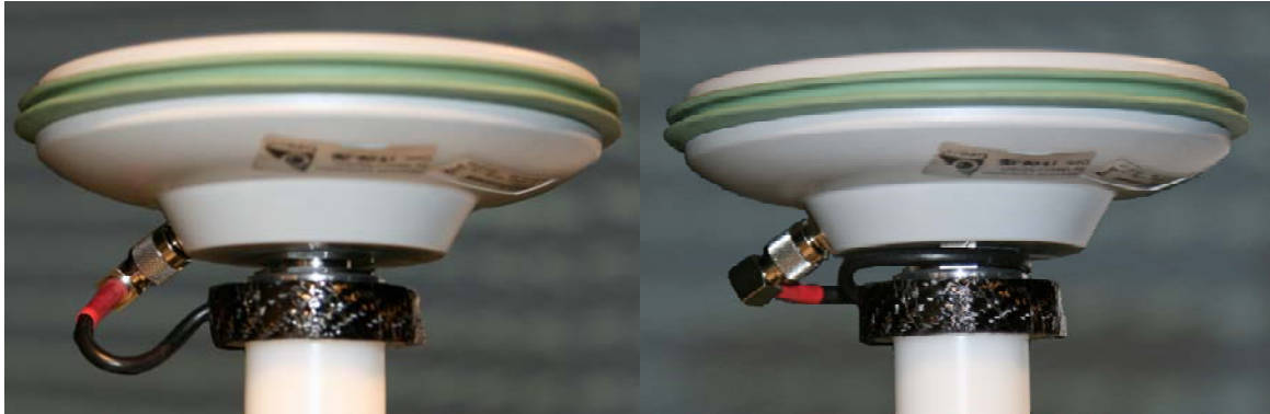
Fig. 7: Differences in cable placement.
